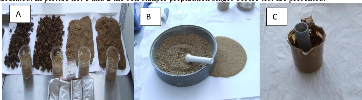
Fig. 1 Soil treatment (A - drying, B - sieving, C – water saturation)
