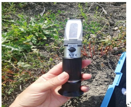
Figure 1. Work stages applied to the buckwheat crop, in the basic apiary in Cornetu (Ilfov county, Romania), for making honey determinations: a) isolation of inflorescences in buckwheat plants, b) empty capillary weighing balance, c) reading the amount of sugar using the refractometer.
